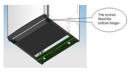
Note: the refrigerator-freezer incline angle less 45  $^{\circ}\,$  .
